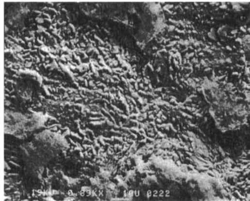
FIGURE 7 A) Scanning electron micrograph of non-corroded area of electroplated zinc substrate. B) Micrograph of corroded area showing altered morphology.
